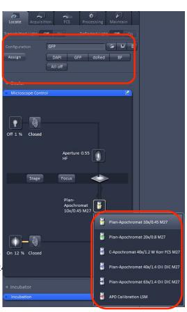
• Use the touchpad RL illumination option or the locate tab "Off" icon to close the shutter.
